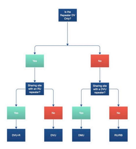
DVU, DVU-R, DMU – 9 MHz channel spacing (Bandwidth 12.5 kHz) RU, RU-R – 7.6 MHz channel spacing (Bandwidth 12.5 kHz) RB – 1.6 MHz channel spacing (Bandwidth 25 kHz)
